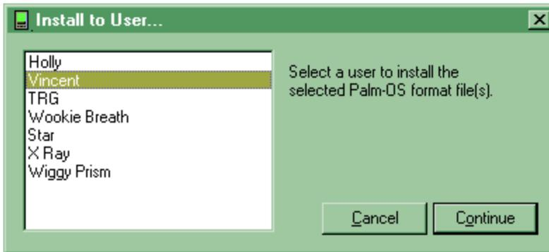
The user selection screen lets the customer choose which Palm unit to install the selected file. Alternatively, TeallInstall can be set up to automatically choose the first Palm user found; useful if only one Palm user is expected on the target computer.
